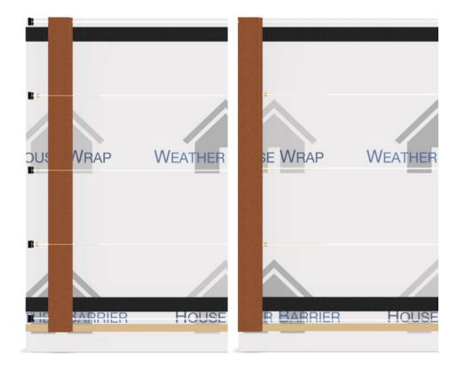
Step 10: Gently tap the bottom of the rainscreen board until it is flush with the furring strip. Fasten the board through the face with 2 screws. You will need to pre- drill the rainscreen board in order to face screw and avoid any splitting. We recommend using a screw and plug system for a seamless look.
