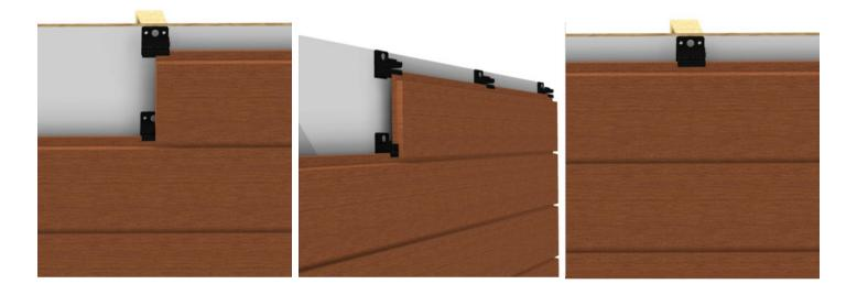
**Step 12:** When you are ready to install your last complete board, screw another course of Cor-A-Vent behind the board. The Cor-A-Vent will sit between your last two rows of clips.
